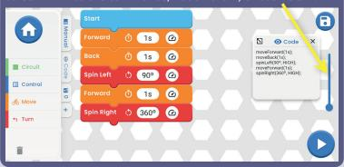
When you enter a command from TURN and click on the 1s time, a window will open where you can set not only the time, but also the degrees of turning (by clicking on Degrees or Time). The degrees are selectable from 0 to 360°.
