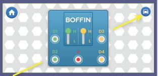
CP has 5 outputs (D1, D2, D3, D4 an A) which are controlled by the app. Outputs D1-D2 and D3-D4 are paired so that each hcontrols a motor in both directions and they can be used to set one of the two levels output voltages, called H (high) and L (low). Output A has a low power output that can control the horn (W1), but cannot control the car's wheel motors. Use the app to control them.
