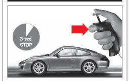
The car programmed to the speed controller will have to come to a stop for at least 3 seconds before the light can be switched on or off by the push of the lane-change-button.
