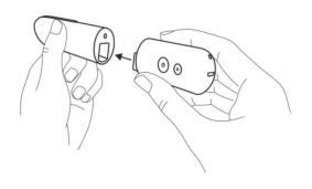
2. Once the battery light turns green, then it is fully charged and you can connect both parts.
