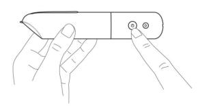
3. When both parts are connected, press the power button and 3Dsimo basic will begin warming up.
