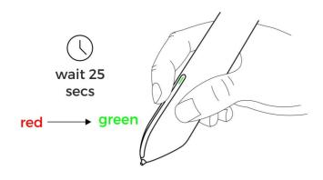
4. Once the front button turns green, then the extruder is heated and ready.
