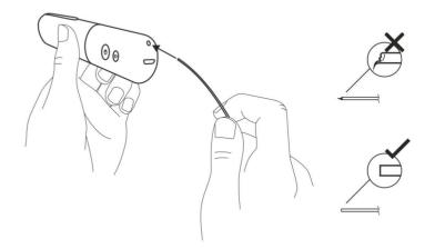
5. Now you can insert a string of PCL material. Make sure that the string is not deformed and its end must be always flat, not jagged. When string is inserted into 3Dsimo basic, hold the front button and gently push the string forward.
