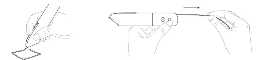
6. String is going to be pulled towards the nozzle and after 8-12 s material will start extruding.
