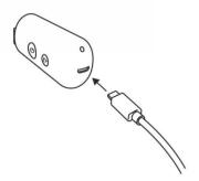
1. We recommend charging the battery after unboxing 3dsimo basic. You can use provided USB cable and plug one end to PC or phone charger and the other one to the back part of the battery.
